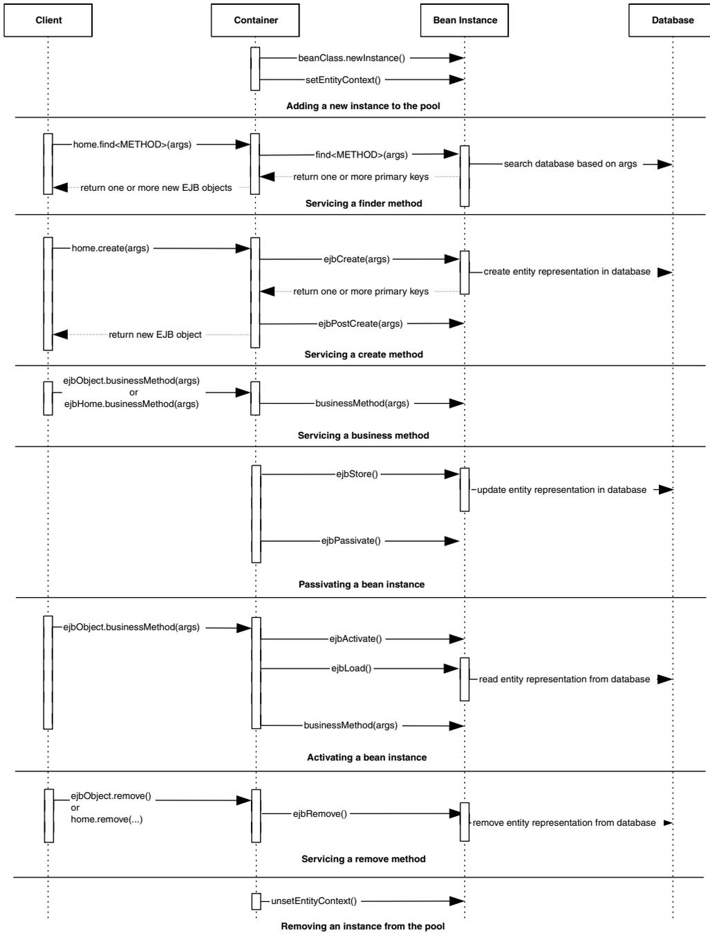
**Figure E.11** Sequence diagram for bean-managed persistent entity beans. For simplicity, the Container object represents all container subsystems, including EJB objects, home objects, transaction services, and so on.
