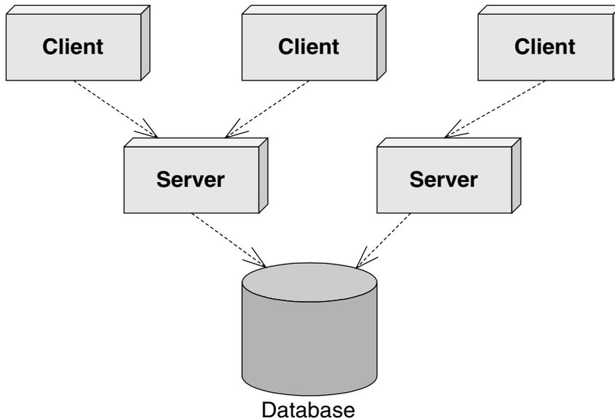
**Figure 1.1** Standard multitier-only deployment.
