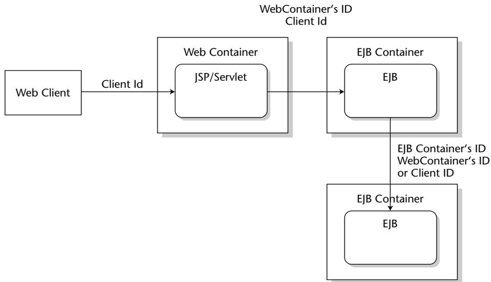
**Figure 13.5** Identity assertion in a call chain.
