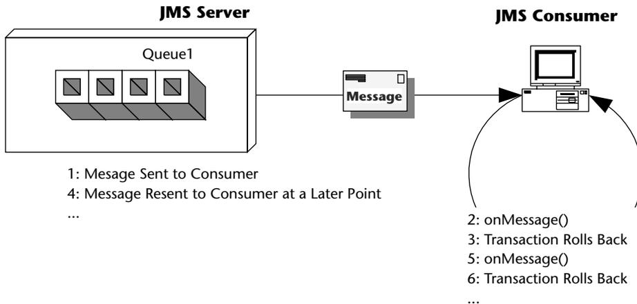
**Figure 9.7** How JMS message-driven beans can cause poison messages.
