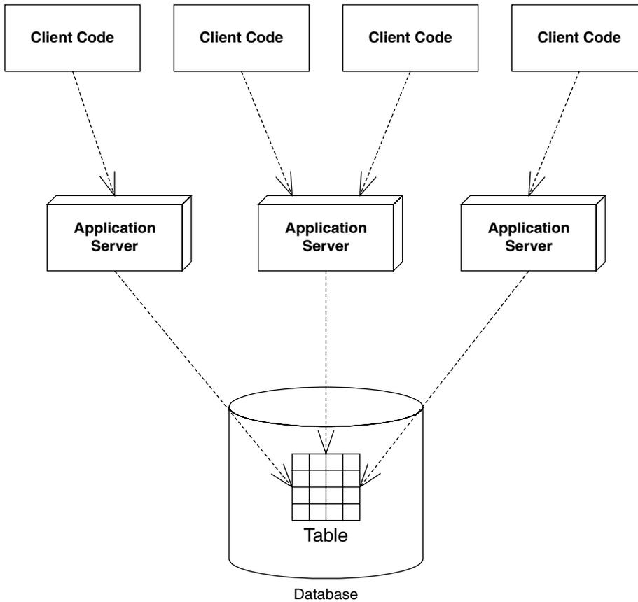
**Figure 12.2** Application servers tied to a single database.
