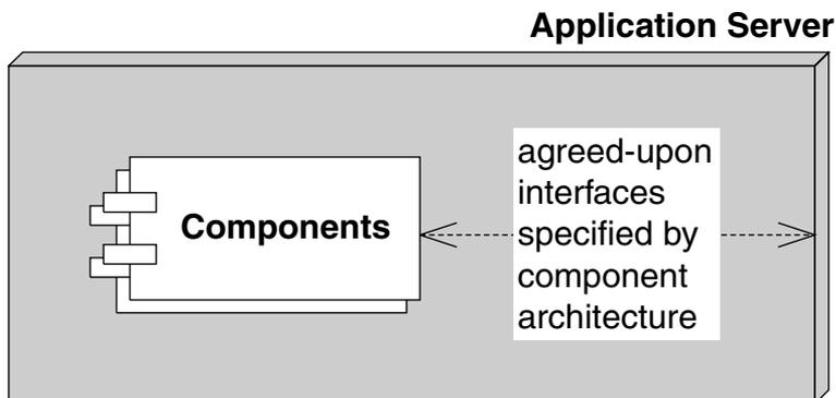
**Figure 1.2** A component architecture.
