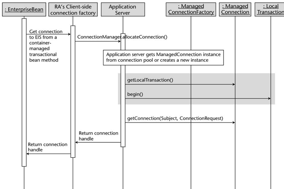
**Figure 17.8** Local transaction management for container-managed transaction.
