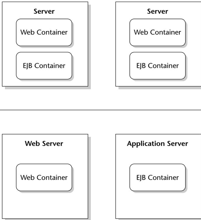
**Figure 19.1** Collocated versus distributed server architecture.
