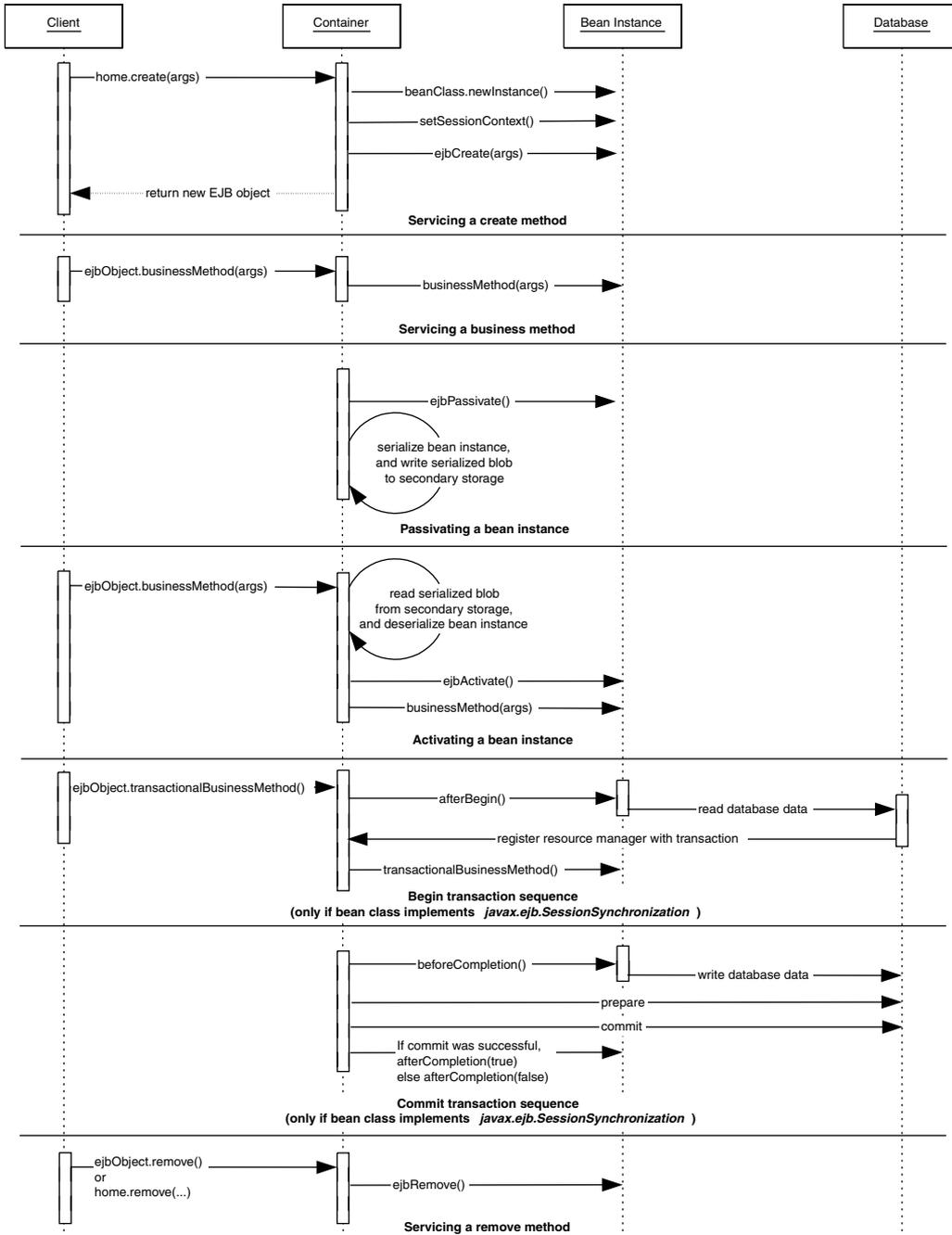
**Figure E.7** Sequence diagram for stateful session beans. For simplicity, the Container object represents all container subsystems, including EJB objects, home objects, transaction services, and so on.
