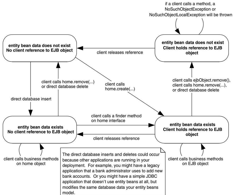
**Figure E.8** The client's view of an entity bean object life cycle.
