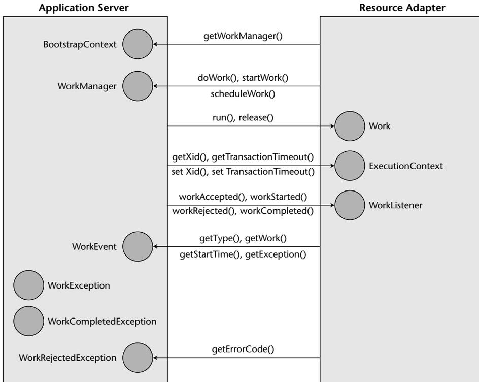
**Figure 17.12** Work management object diagram.
