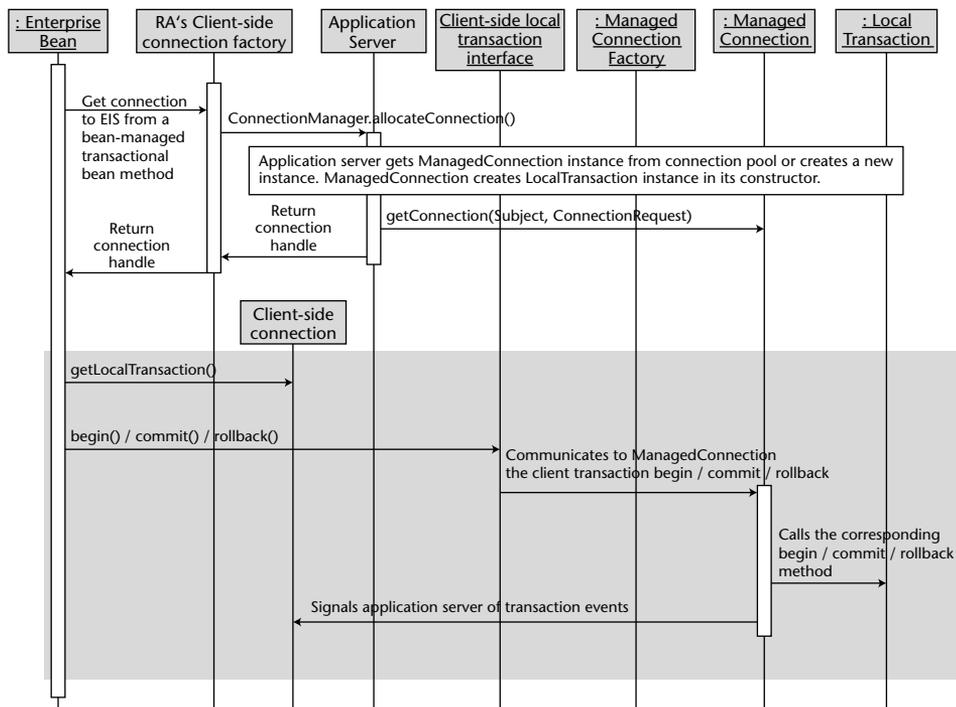
**Figure 17.9** Local transaction management for client demarcated transaction.
