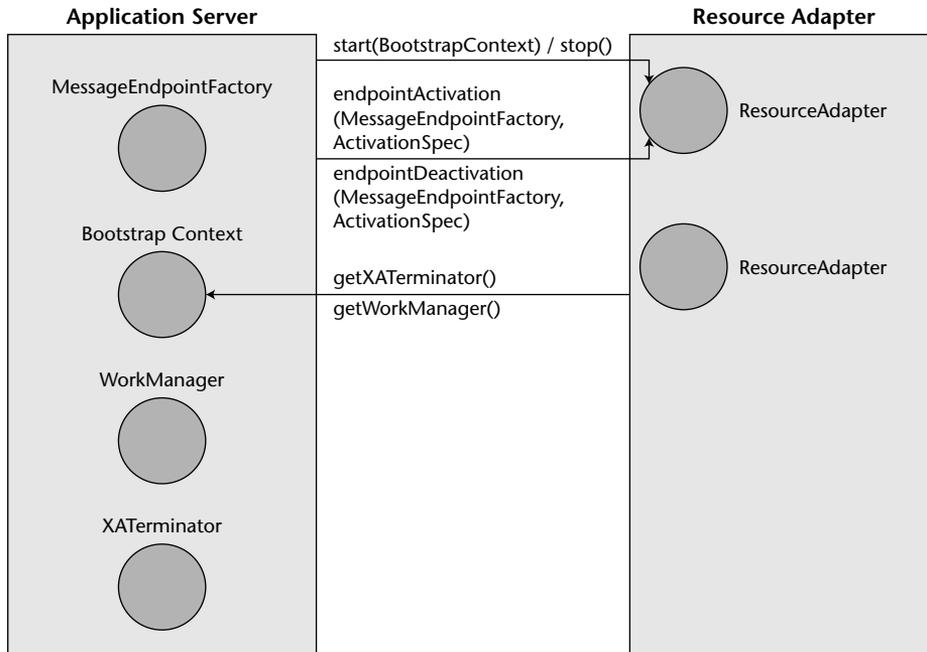
**Figure 17.4** Life cycle management object diagram.
