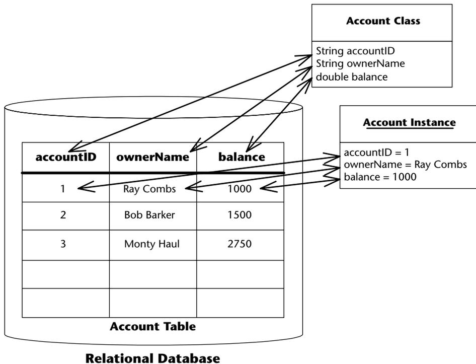
**Figure 6.2** An example of object-relational mapping.
