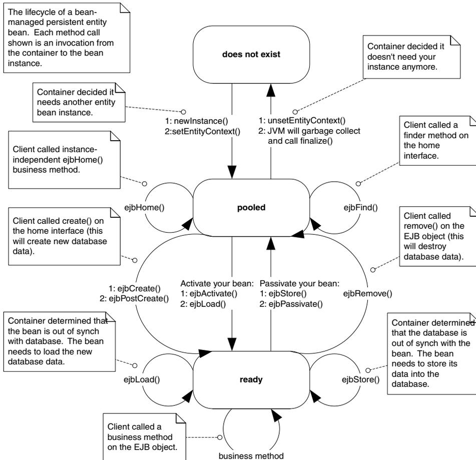
**Figure E.9** The life cycle of a bean-managed persistent entity bean. Each method call shown is an invocation from the container to the bean instance.
