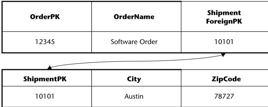
**Figure 15.2** A possible one-to-one cardinality database schema.
