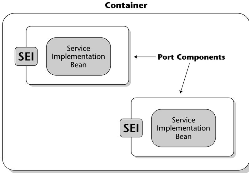
**Figure 5.2** EJB container with port components.
