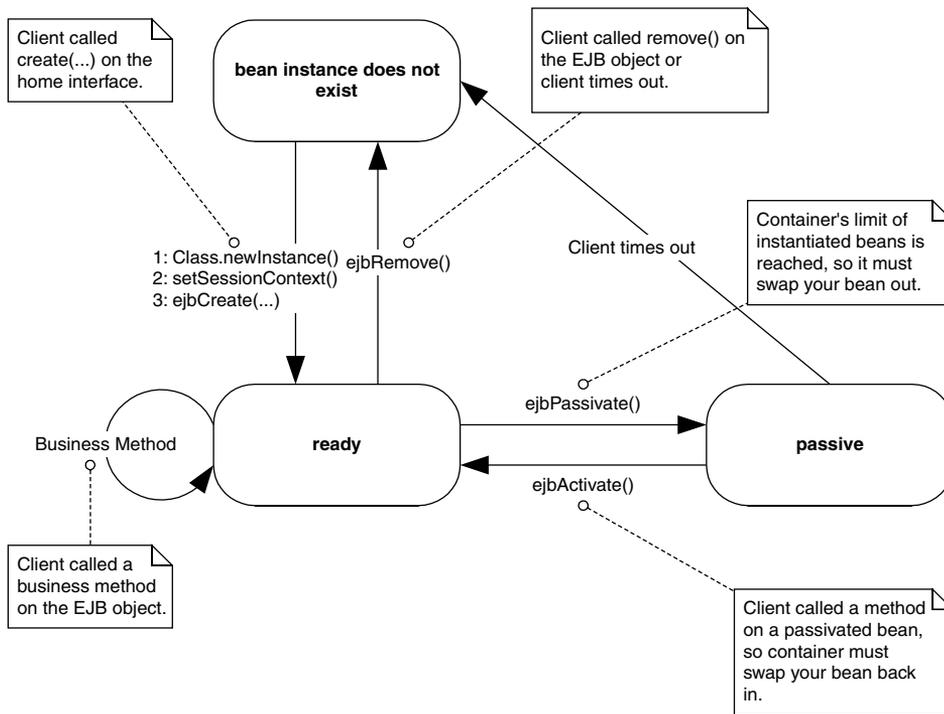
**Figure E.5** The life cycle of a stateful session bean (does not implement *javax.ejb.SessionSynchronization*). Each method call shown is an invocation from the container to the bean instance.
