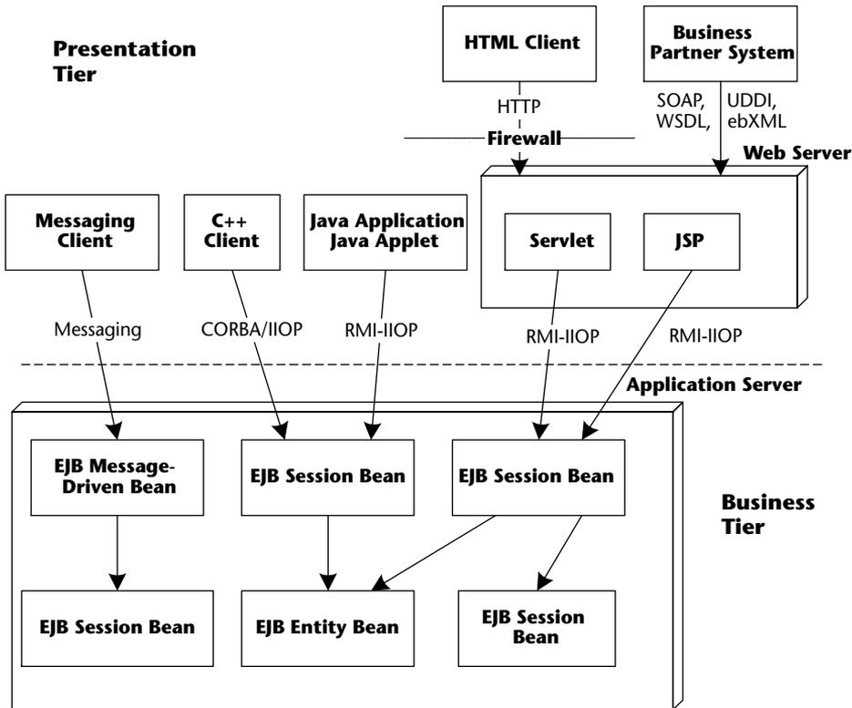
**Figure 2.1** Clients interacting with an EJB component system.
