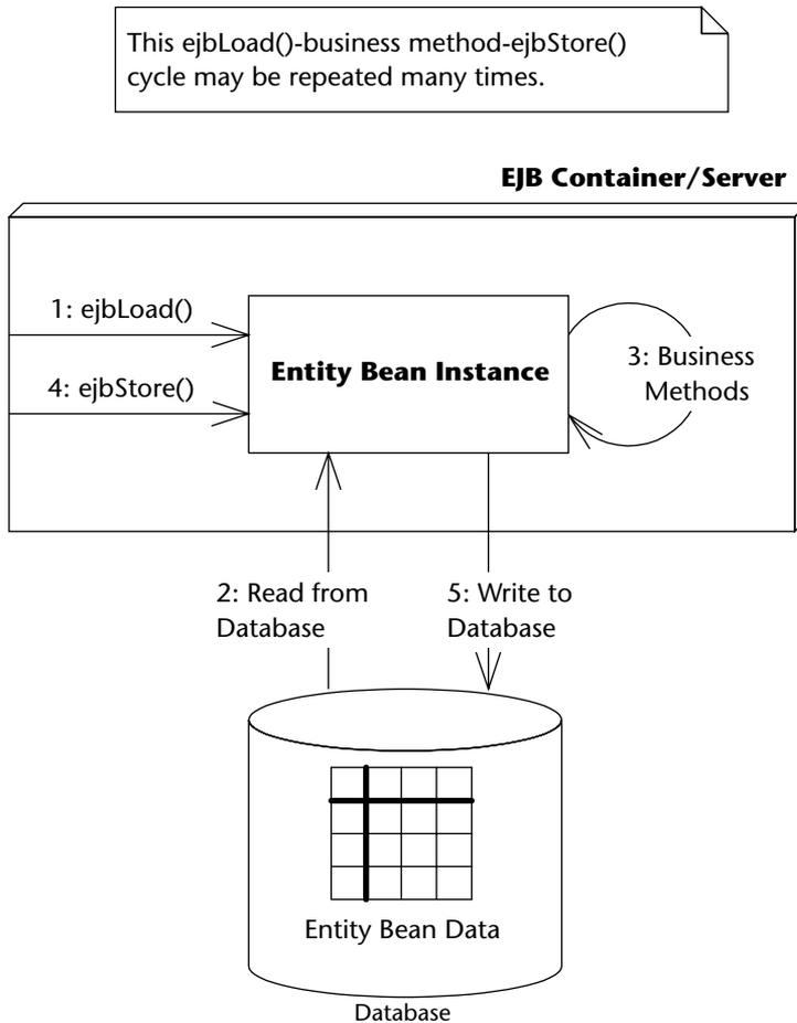
**Figure 6.3** Loading and storing an entity bean.
