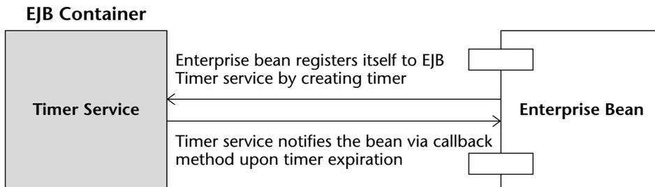
**Figure 14.1** Interaction between the timer service and EJB.
