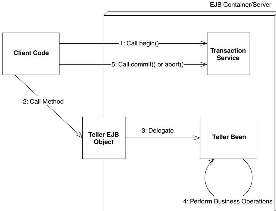
**Figure 12.7** Beans with client-initiated transactions.
