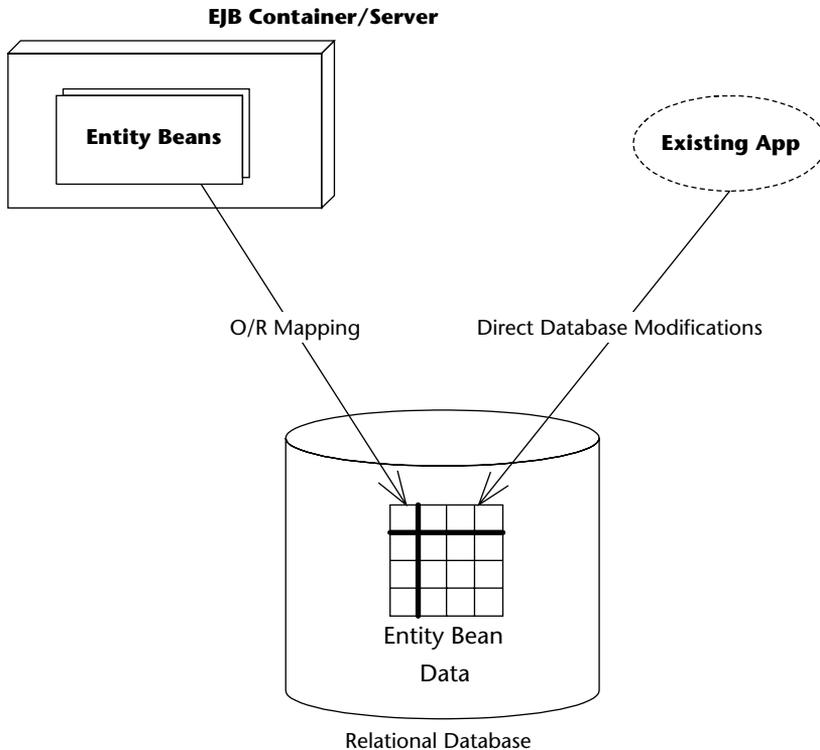
**Figure 6.8** Modifying an entity bean's database representation manually.
