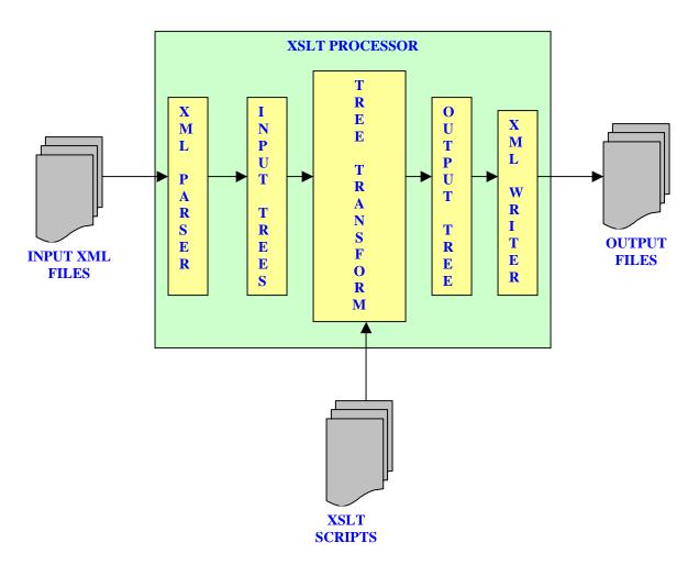
Figure 2: XSLT based document generation process
