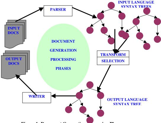
Figure 1: Document Generation Processing Phases
